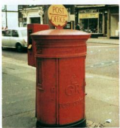
No. 18. This oval shaped pillar box was introduced experimentally in 1932 to provide the means of purchasing stamps at the point of posting. The stamp machine can be seen incorporated into one end of the box, whilst the posting aperture is at the other end. The box was made in two sizes by Derby Castings Ltd, this one being of the larger type. Very few of these boxes can still be found and the one shown is at South Levenshulme TSO, Stockport Road, Manchester.
